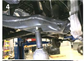
e. Loosen and remove the lower control arm Cam bolts using a 21mm and 24mm socket and wrench. Be careful and ensure the spindle is supported properly, either with a jack or stands. (PHOTO 5)
